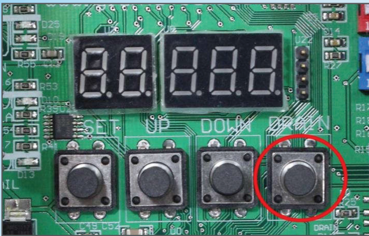
Press and hold “DRAIN” key to start drain pump
