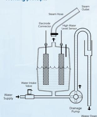
When using tap water, supply water conductivity should range between 125 and 1250 µS/cm. This electrode steam humidifier uses tap water to produce steam; once water fills the cylinder, the electrode activates a current that heats and boils the water to create steam.
