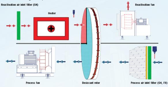
Note: depending on specific requirement, electric heater can be replaced fully or partially by condenser coil for better COP.
